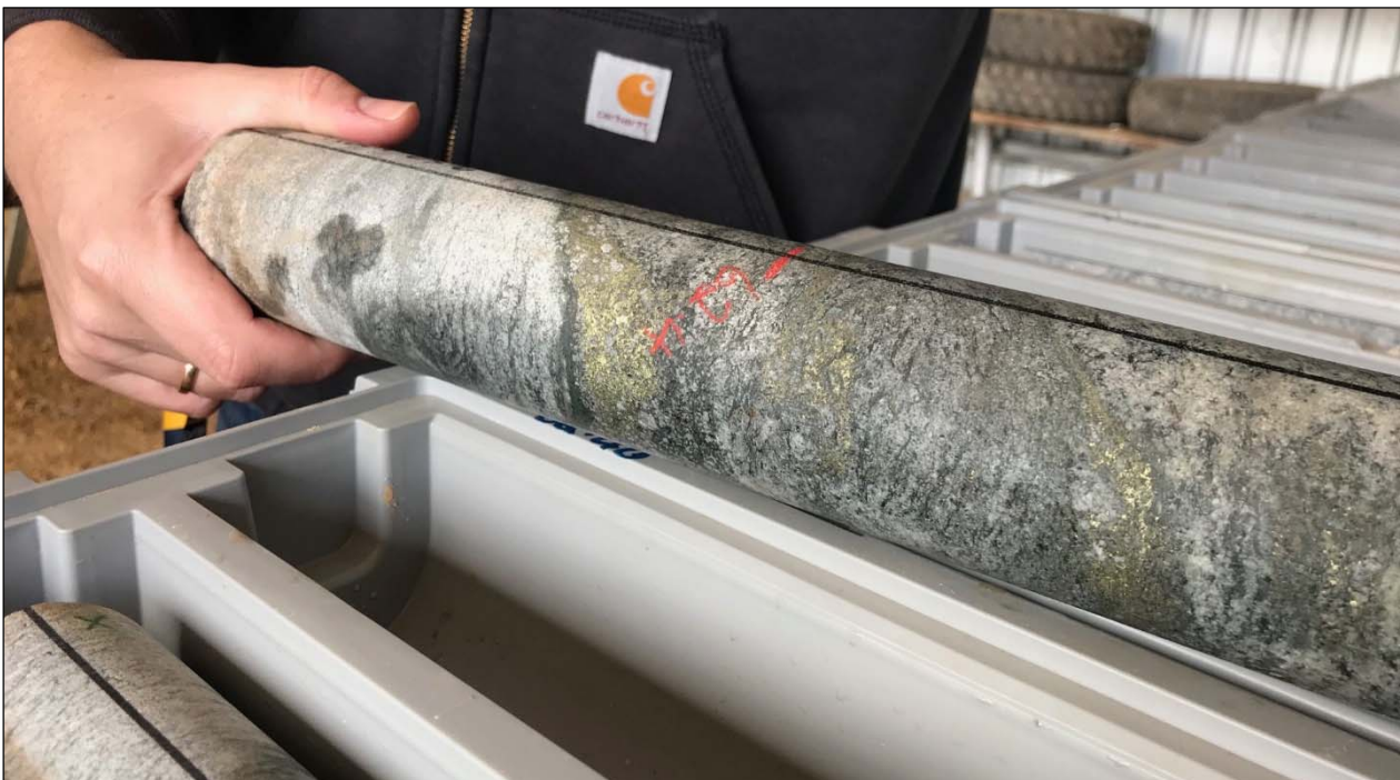
Figure 1: Chalcopyrite mineralisation from higher grade domain within Bindi West resource, intersected in diamond drill core from hole 18CAD001 at 62m depth.
