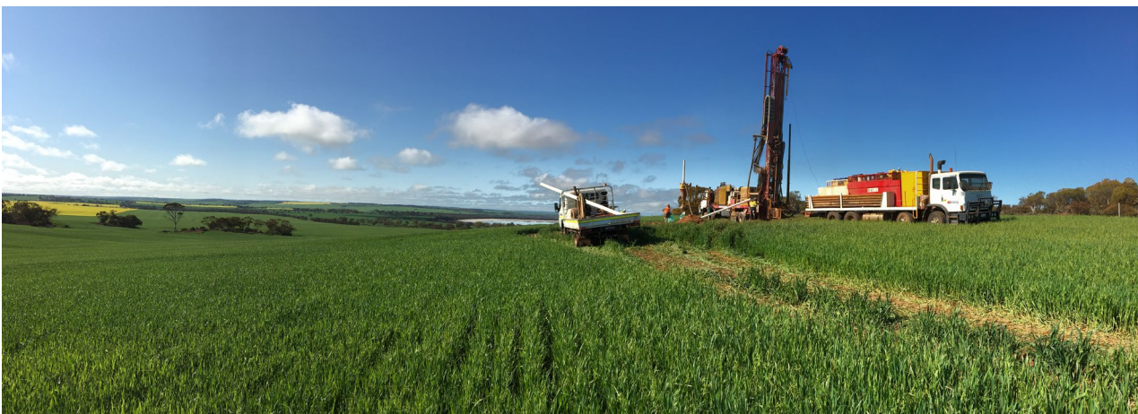
RC percussion drill rig and support vehicles at the Ninan Prospect, Caravel Copper Project
