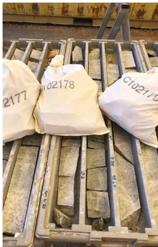
Figure 31: Diamond core for metallurgical testwork.
