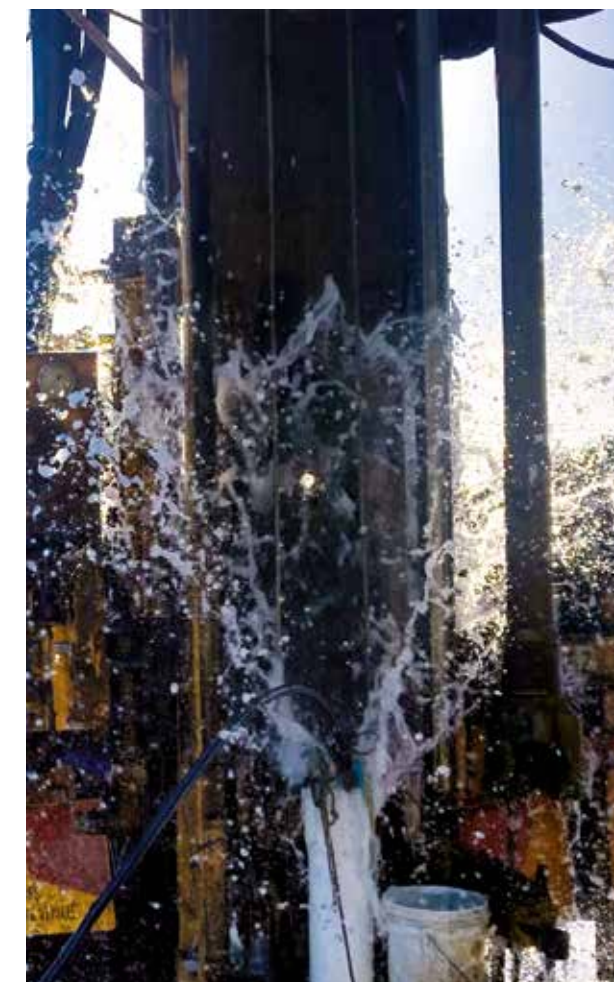
Figure 36: Water pump testing in progress at potential borefield area.
