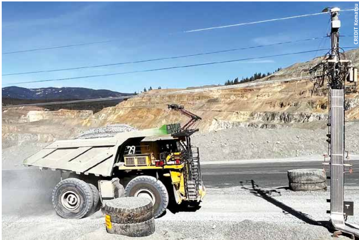
Figure 40: Autonomous mining vehicle on dedicated haul road.
