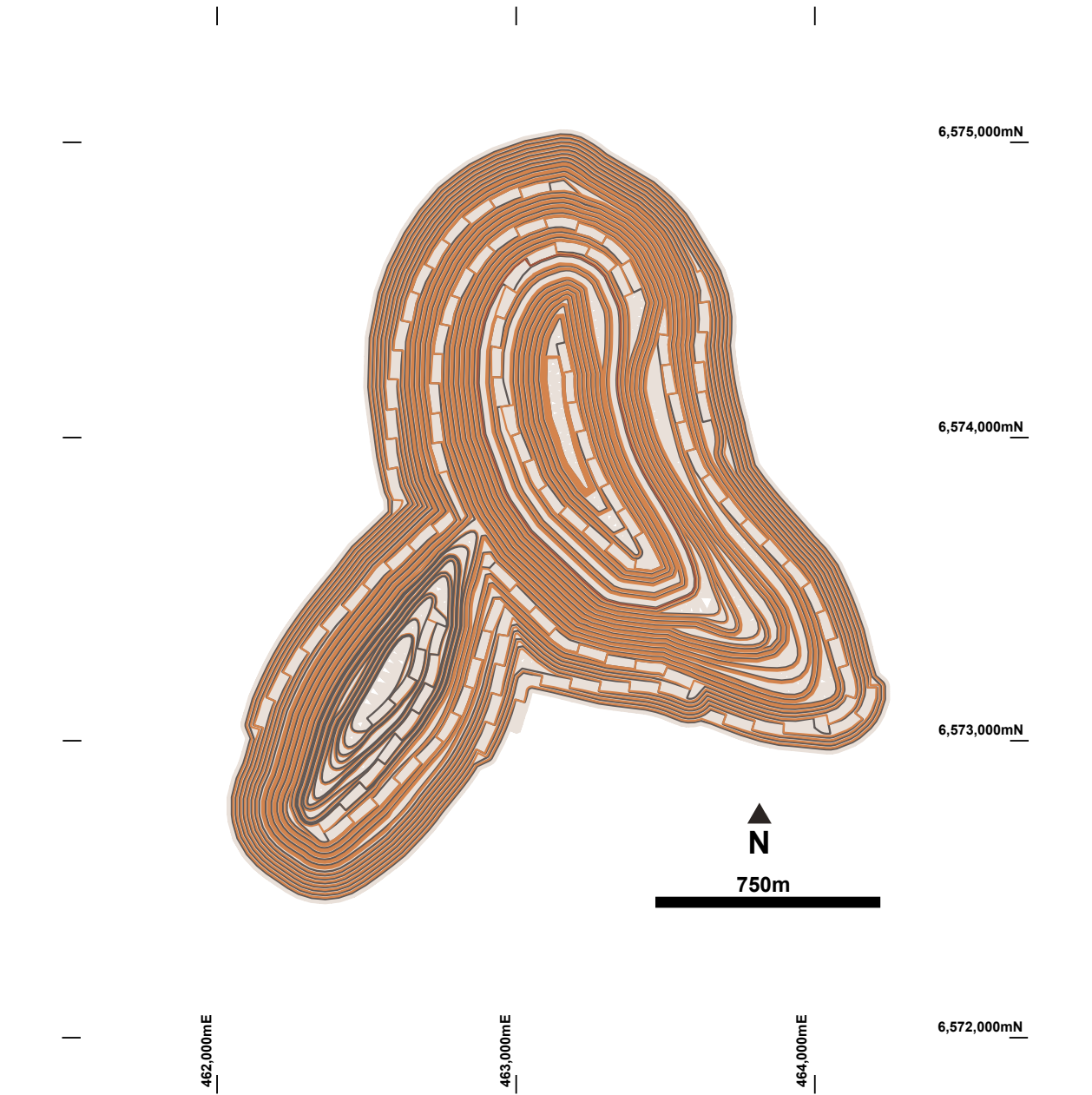
Figure 21: Bindi Pit design for stages 1 to 5.
