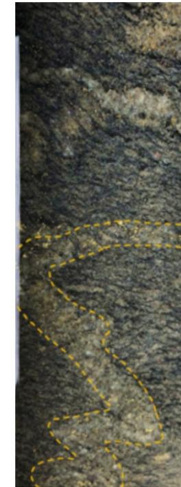
Figure 5. Drill core showing late folding of early foliation and veins.
