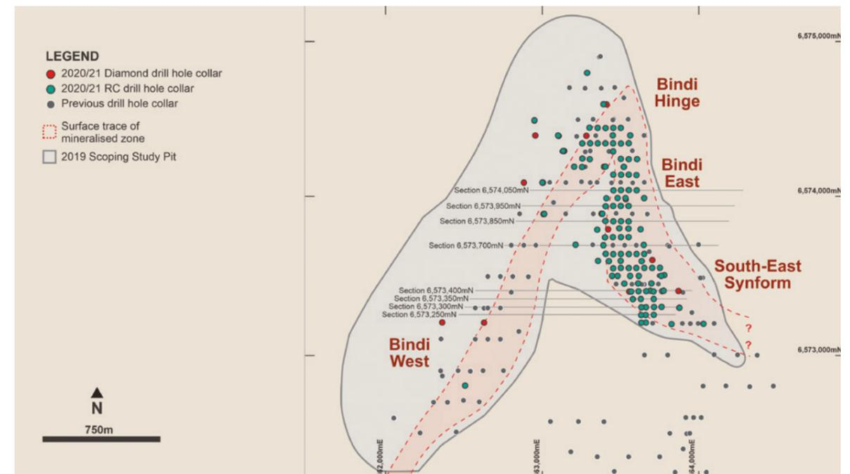
**Figure 9: Drilling status plan of the Bindi copper deposit showing the locations of 2020/21 drill hole collars and previous drill collar locations.**
