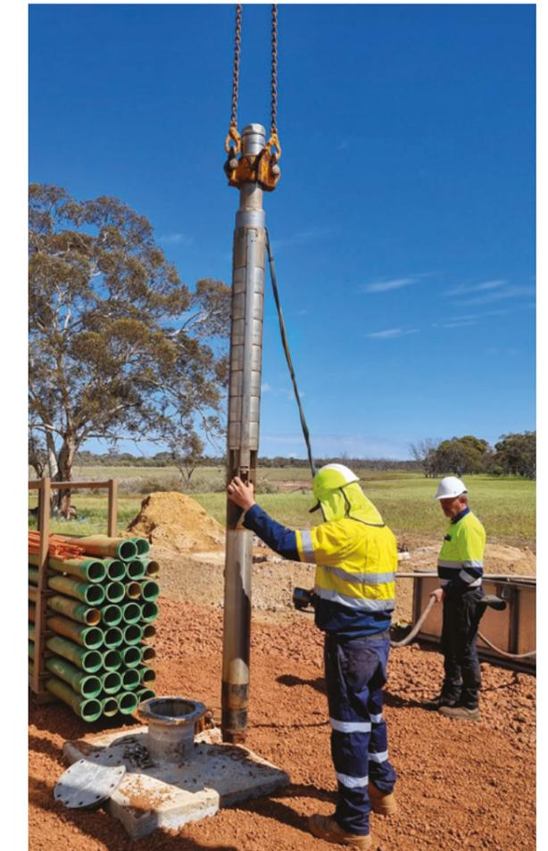
Above: Pump testing at potential borefield.
