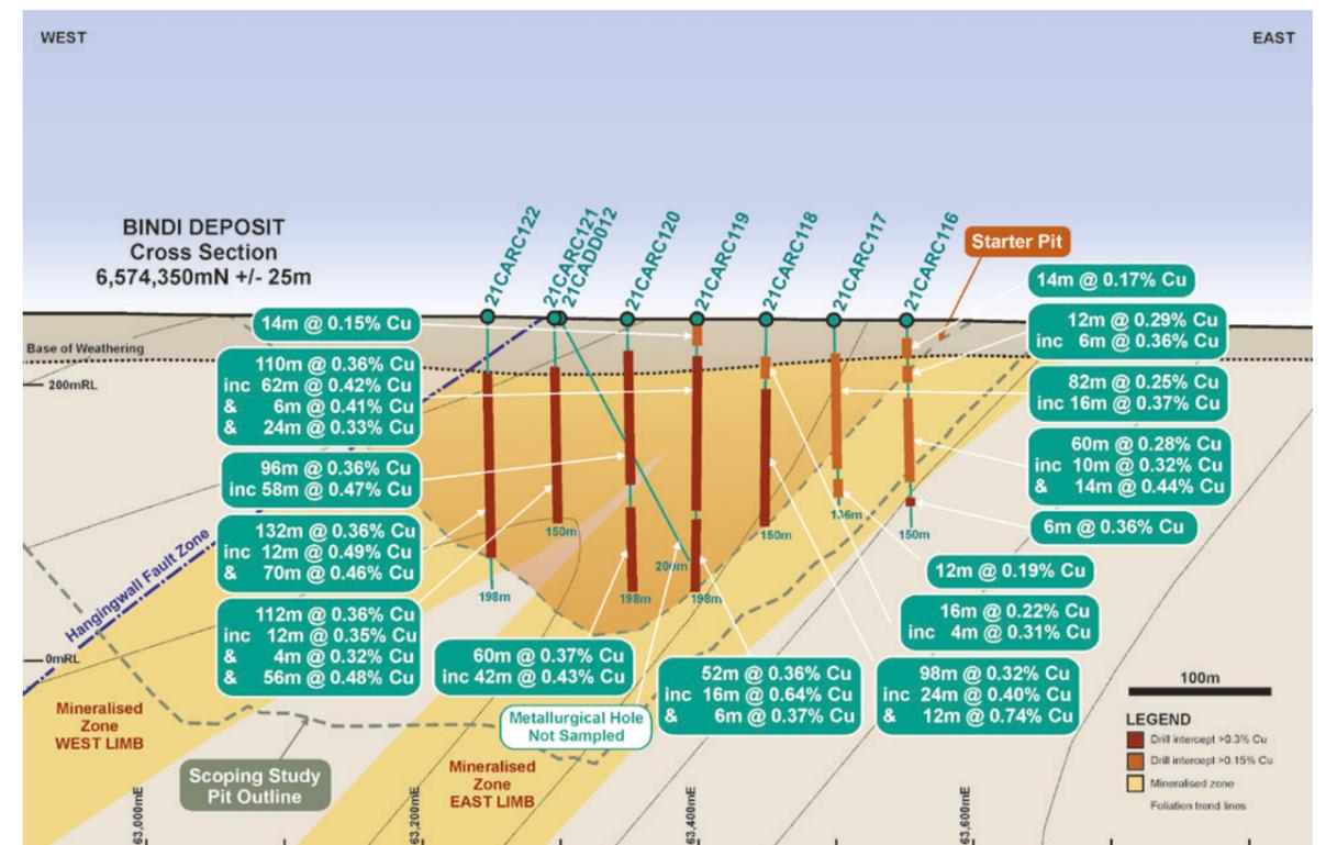
Figure 12: Cross section through Bindi Hinge Zone showing drill intercepts and structural interpretation.
