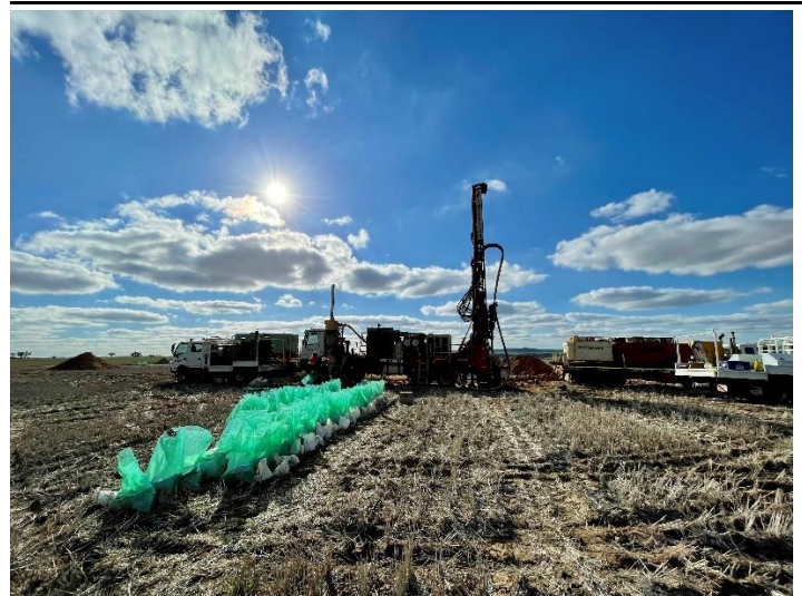
Figure 50: Close up of RC drilling
